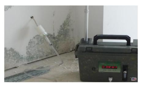
In this brand-new building, mould developed on walls even before painted. The client asked to test cavities and recommend correct protocols. The cavity was completely contaminated, and all walls had to be removed back to framing
